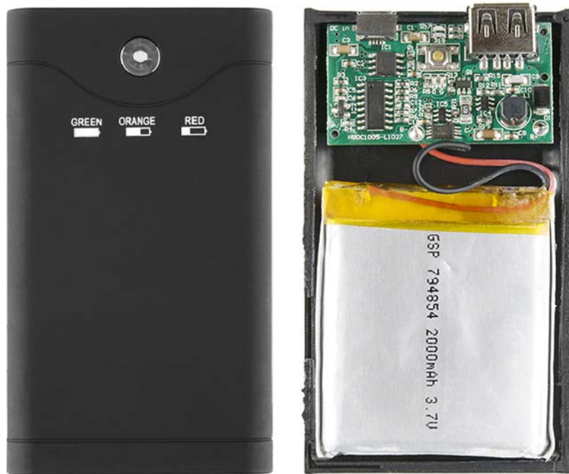
Figure 10 – Power Control Board and Battery inside the SparkFun USB Battery Pack - PRT-11359
