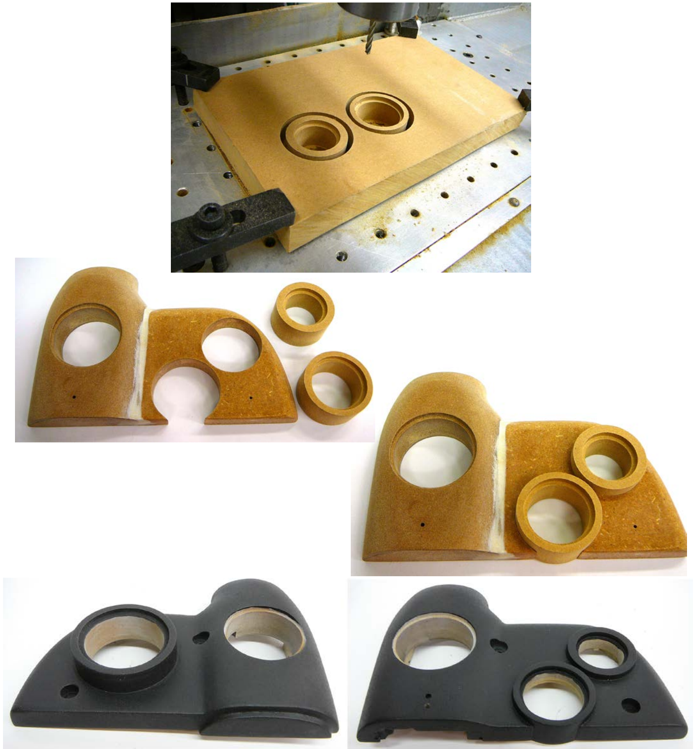
Figure 38 – Steps involved in making the side covers. Top - CNC machining the cylinders, Center – Gluing the cylinders, Bottom – Finished covers painted with Rust-Oleum 7220-830 Textured Black Enamel .
