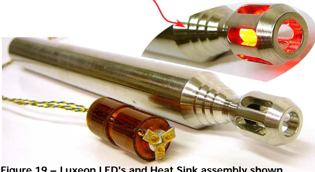
Figure 19 – Luxeon LED's and Heat Sink assembly shown approximately where they are fitted when installed toward the front of the turned Aluminum barrel.
