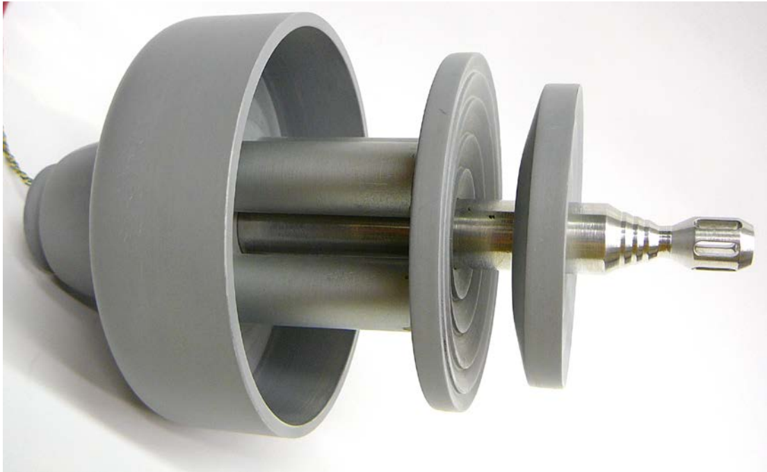
Figure 56 – The Beam Concentrator Assembly after painting with grey RustOleum primer 2081 prior to application of the rectangles.
