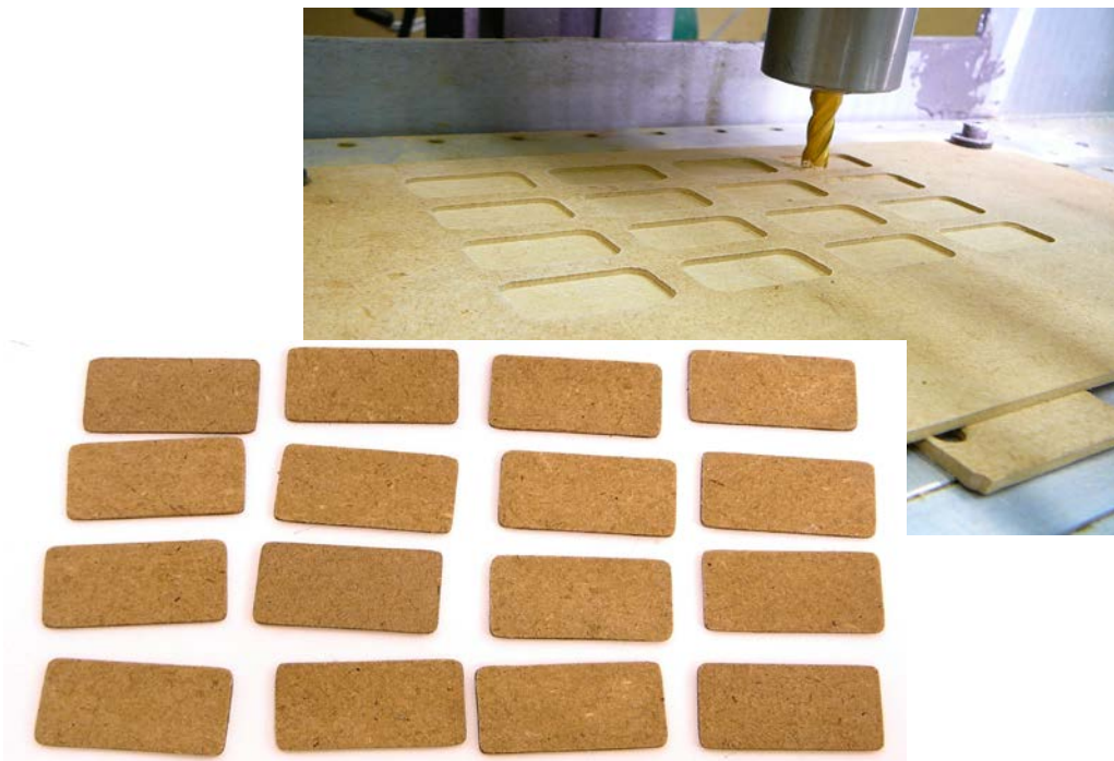
Figure 55 – The beam concentrator cup assembly consists of 3 details, 4 disk support rods, 12 cup outer diameter rectangles and the cup. This photo shows the 0.125 inch MDF stock being thinned down to 0.060 inch as part of the CNC machining operation of the rectangles.
