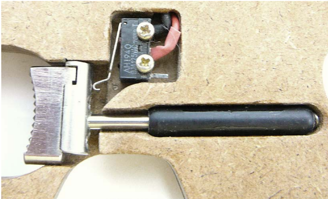
Figure 24 – The trigger and microswitch that it actuates, there's a small coil spring inside the black plastic tube that returns the trigger when it's released.
