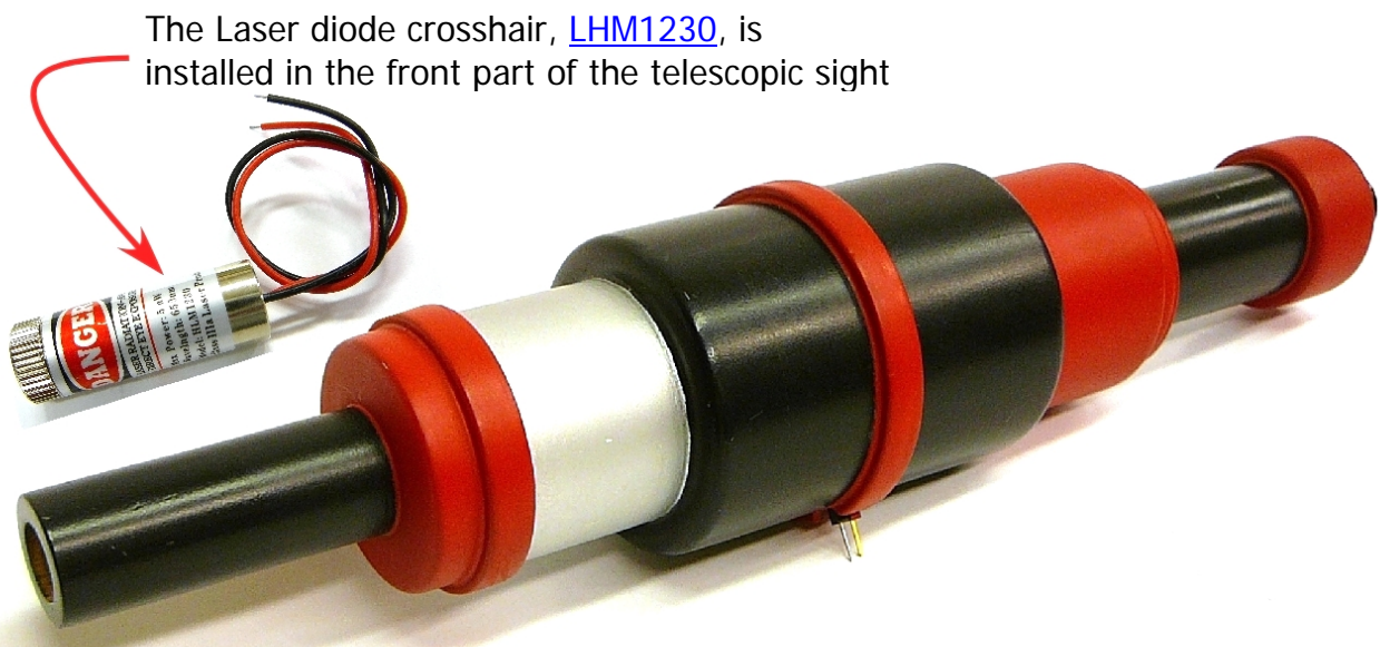
Figure 23 – The telescopic sight is fitted with a 5mW 650nm Red Laser diode crosshair, LHM1230. The crosshair Laser draws 13mA and is driven directly by the Arduino, it's connected to digital pin 6.
