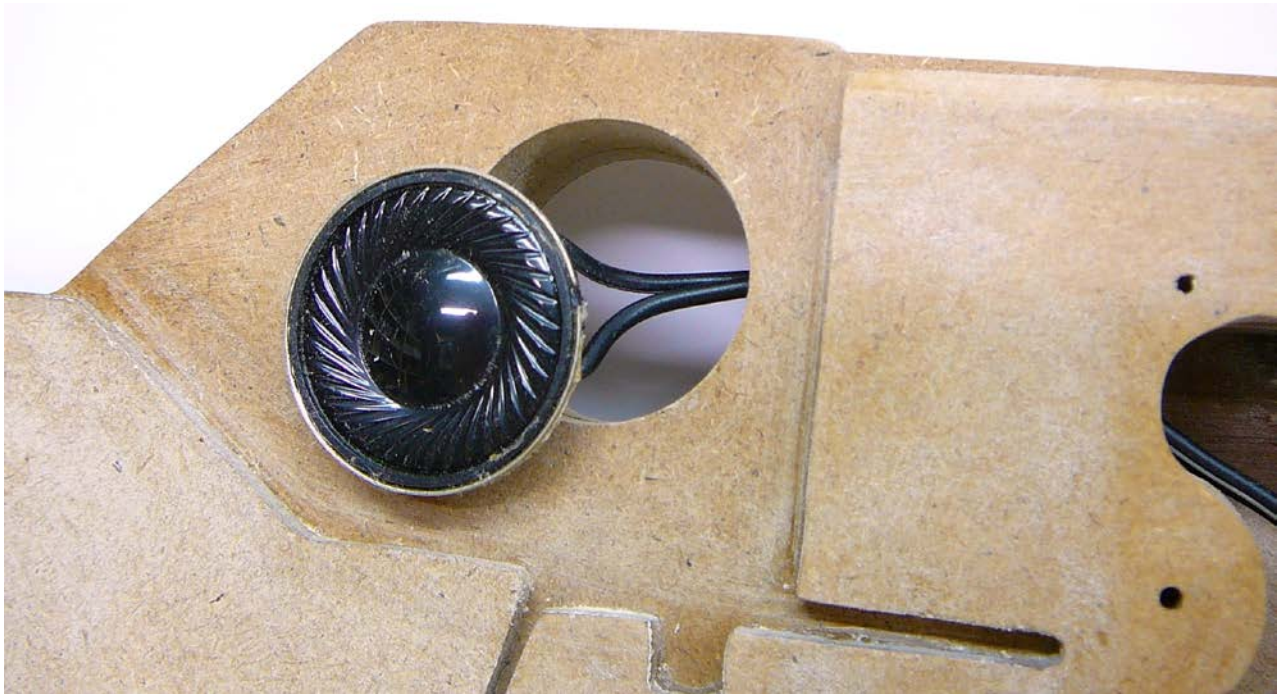
Figure 21 – One of the speakers about to be mounted into the mating hole in the gun body.
