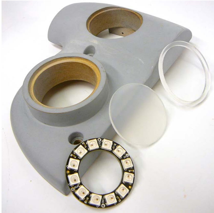
Figure 33 – The 12 pixel NeoPixel ring PCB assembly from Adafruit is mounted in the left side cover assembly under a diffuser disk and a clear lens.
