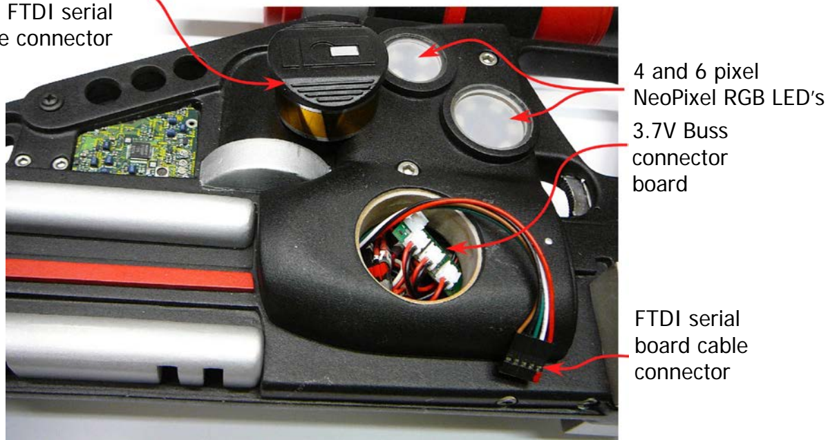
Figure 15 – Breakout board cable connects OSEPP Pro Arduino processor board to FTDI serial to USB board.
