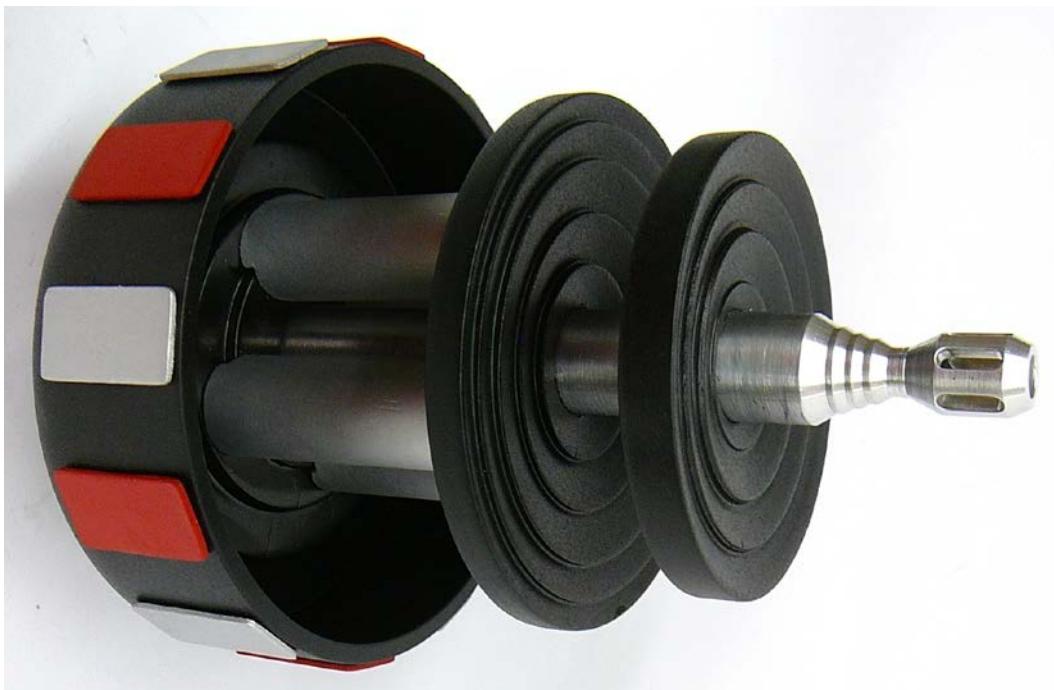
Figure 57 – The Beam Concentrator Assembly after application of the rectangles and finish paint with Rust-Oleum 7220-830 Textured Black Enamel.
